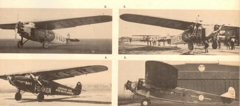
engineers had predicted. Radial engines were eventually wing-mounted, but not until after NACA had smoothed out the airflow with its new cowling, introduced in 1929. The second Ford trimotor had the side engines under the wing and in the long run proved to be a more successful design than the Fokker, thanks mainly to its all-metal construction.
