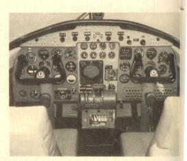
Dual nav/com equipment with two 360-channel transceivers, two 100-channel nav receivers with course indicators, marker beacon/glideslope, DME, and transponder are part of the Hawk's basic IFR avionics system. Numerous optional items also are shown here. Photo by Aero Commander
